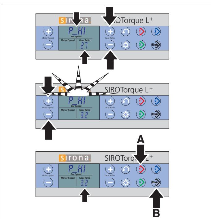
To be able to fully use the control range of the pneumatic speed controller foot switch, the compressed air pressure in bar which is present at the air supply hose outlet should be set in this menu. If you want to reach the preset maximum speed already before having pushed the pedal fully down, you can reduce this pressure.
