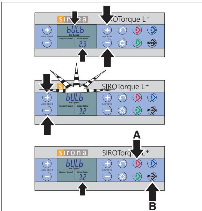
If you feel that the cavity is over-illuminated or under-illuminated by the instrument light, you can adjust the lamp voltage.
